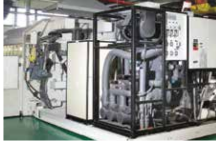
High Vacuum Web Coating Process
