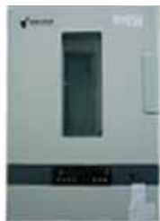
Thermo-hygrostat reliability measurement of temperature and humidity
