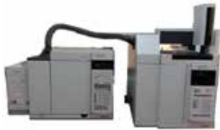
GC-Mass residual solvent measurement
